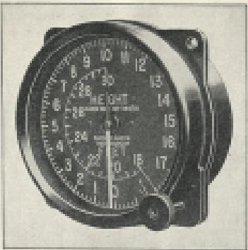
2. The Mark XVII altimeter fitted in Elementary Flying Aircraft.
