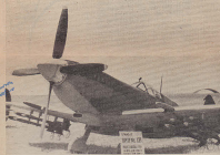
This Supermarine Spitfire R.P. Mk. XVI, fitted with Mark VIII zero-length rocket installations, is seen here with eight rockets under the wings.
