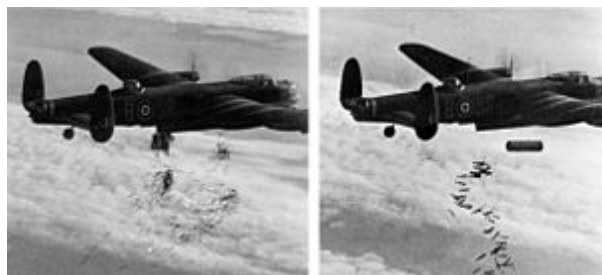
Lancaster B I NG128 dropping its load over Duisburg on 14 October 1944. The aircraft is carrying Airborne Cigar (ABC) radio jamming equipment, as shown by the two vertical aerials on the fuselage.
