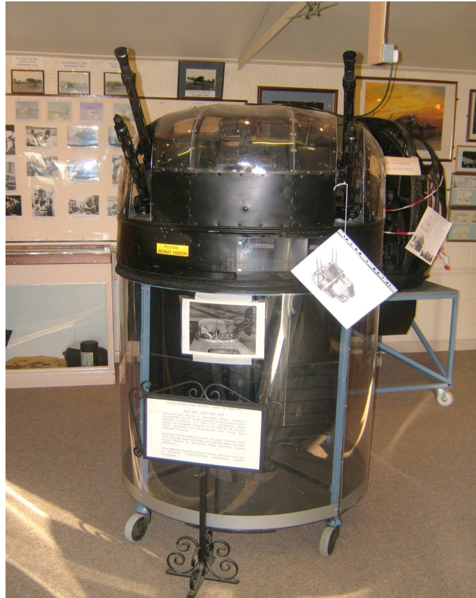
A Boulton Paul MkVIII Type 'A' Turret. Ref No. 50A 108-109 Recovered from a Handley Page Halifax, Serial DK116 of 1660 Heavy Conversion Unit, which crashed on the 15 th October 1944 after an engine failure at 12,000 Ft. It struck high ground on Grapstone Fell, near the Kielder Forest. During restoration work, it was found that the turret was actually an earlier MkII of the type fitted to Boulton Paul Defiant night fighters. The MkVIII modifications were carried out by a French engineering company called S.A.M.M.
