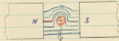
By interaction of the magnetic field of the conductor & the initial field, the conductor moves the direction being given by Fleming left hand rule.
